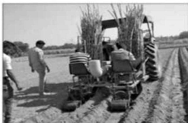
Fig.1. IISR Deep Furrow Sugarcane Cutter Planter and Trench Planter
